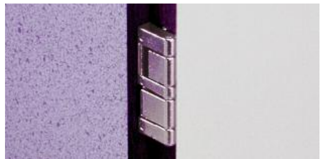
Object hinge (Fa. Prämeta) for Compact doors panels, door thickness 10 -13 mm. Single axis pivot point.
