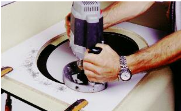
2. Rebate from the underside of the Compactforming Element with a rod miller or CNC machining centre.
